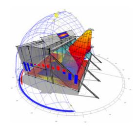
A technique which builds computer models for analysis & focuses on energy consumption, life cycle analysis of energy related equipment/systems and the absolute cooling/heating loads. It takes into consideration of building architecture, orientation (sun path analysis), shading from adjacent structures, systems/equipment, automation & controls along with exact operation philosophy
